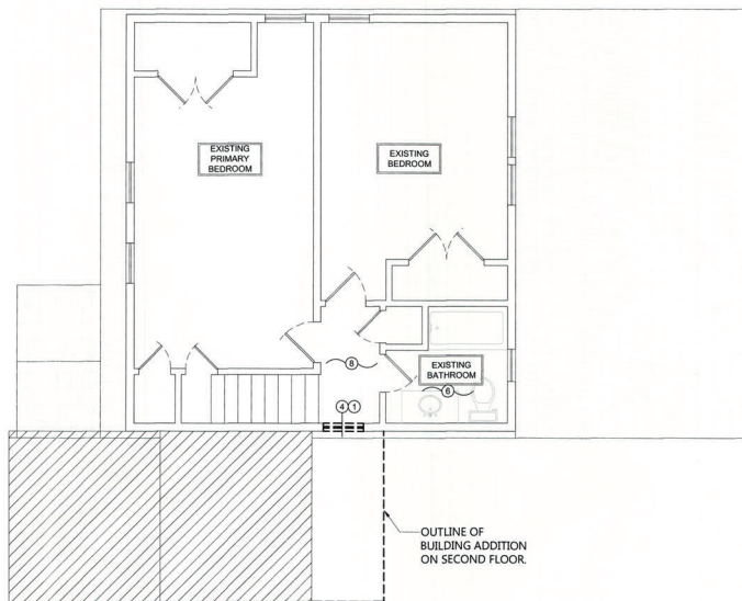
1 DEMOLITION SECOND FLOOR PLAN A-02 SCALE: 1/4" = 1'-0"
